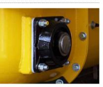
Heavy-duty ball bearings Four bolt flanged bearing
