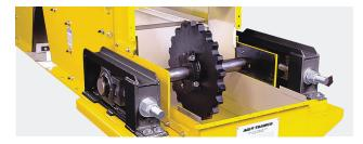
Double-Life and Walking Tooth sprockets are available. Walking Tooth sprockets are only available in 6" pitch chain. However, Double Life sprockets are applicable for any pitch chain with an even number teeth.
