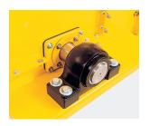
Heavy-duty, long life pillow block roller bearing Packing gland shaft seal
